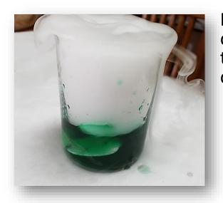
Place dry ice in a cup. Add different temperature water to measure how quickly the dry ice sublimates.
