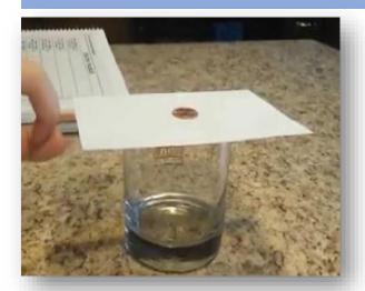
Place a card on top of a cup. Place a penny on the card. Flick the card away. The penny will drop into the cup.
