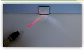
Cast a beam of light with a laser pointer or a flashlight onto a mirror. Use the mirror to reflect the light into different directions.
