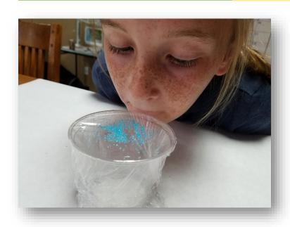
Cover a bowl with plastic wrap. Put rice or sprinkles on the top. Hum next to the bowl. The salt/sprinkles will move around.
