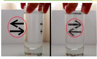
Fill a glass or clear plastic cup with fresh water. Draw an arrow on a piece of paper. Move the paper behind the glass/cup. The arrow will change direction.
